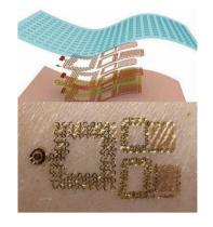
An ultrathin, stretchable device capable of soft lamination onto the surface of the skin for wireless measurements of dielectric and surface strain properties is presented. The device uses LC resonators with capacitive electrodes to qualify the skin properties, and is capable of conformal and spontaneous skin integration.
