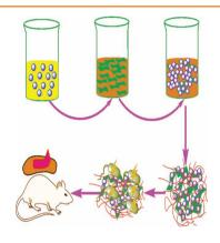
A novel application range of graphene hydrogel in wound dressing is exploited. The hydrogels are composed of Ag-graphene composite, AA, and BIS. When the mass ratio of Ag to graphene is 5:1, the hydrogel (Ag5G1) shows strong antibacterial activity, large swelling ratio, excellent biocompatibility, and good extensibility, and it can significantly accelerate the healing rate of artificial wounds in rats.
