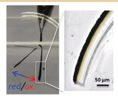
Durable, biocompatible materials capable of controlled movements are sought after for a variety of drug delivery, surgical, and tissue engineering applications. Methods to synthesize films composed of an interpenetrating network of the biopolymer silk fibroin and poly(pyrrole) are described, and the ability of these materials to function as electromechanical actuators in a biologically relevant environment are demonstrated.
