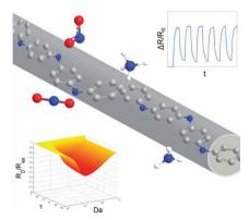
Electrospun polyaniline fibers are fabricated and evaluated as chemiresistive gas sensors. The fibers exhibit remarkable changes in measured resistances for ammonia and nitrogen dioxide sensing, with short characteristic response times. A time-dependent reaction-diffusion model is used to extract physical parameters from fitting experimental data, and to illustrate the selection of optimal material design parameters for gas sensing by nanofibers.
