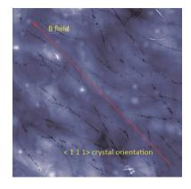
2D-X-ray diffraction analyses of aligned magnetotactic bacteria reveal [111] and [100] fiber textures along the chain direction as a function of cell species. The [100] axis appears unfavorable because it represents a magnetic hard axis in magnetite. Calculations show how this can be turned into an effective easy axis for a given particle elongation.
