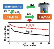
A novel hexagonal Li<sub>2</sub>MgSi is successfully synthesized through a hydrogen-driven chemical reaction technique, which exhibits significantly improved cycling stability with respect to that of Mg<sub>2</sub>Si as an anode material for Li-ion batteries. Ball milling induces a polymorphic transformation of Li<sub>2</sub>MgSi from the hexagonal phase to the cubic phase and further improves the electrochemical lithium storage properties.
