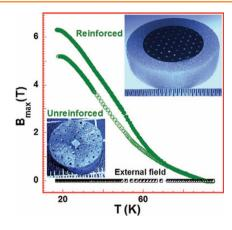
High-performance YBa<sub>2</sub>Cu<sub>3</sub>O<sub>7-δ</sub> bulk superconductors with improved reliability and thermal transfer ability are fabricated in short time. The approach taken here is based on the insertion of a metal wires network into the holes of YBa2Cu3O7-8 drilled single grains progressively annealed at high temperature under oxygen pressure. The achieved microstructure is pore-free and crack-free, and the thermal exchange markedly fosters inside the superconductor.
